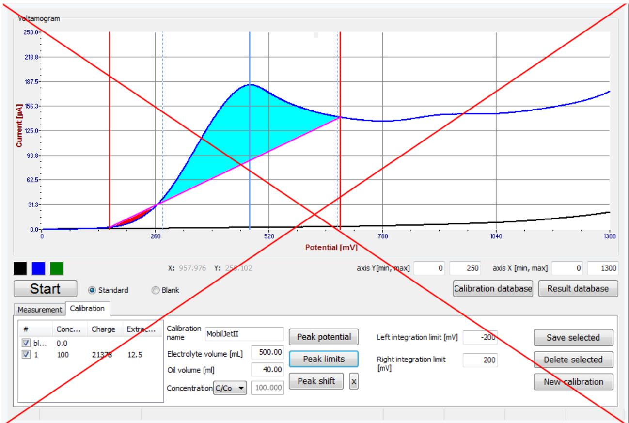
Figure 15: An example of incorrect setting of the peak limits
