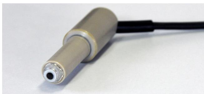
Figure 3: Electrode system of Aditest AP
