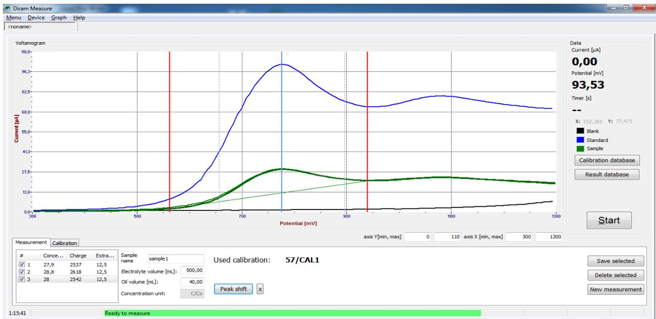
Figure 12: Results for the electrolyte - **Blank** (black curve), **Standard** (blue curve) and three times measured **Sample** (green curves).
