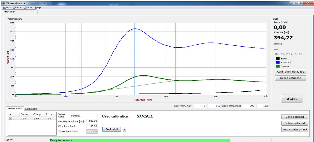
Figure 10: The results for the electrolyte - **Blank** (black curve), **Standard** (blue curve) and **Sample** (green curve).
