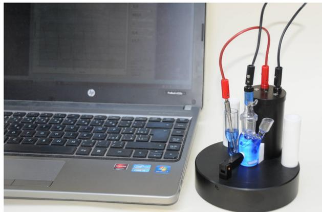
Diram s.r.o. offers two possibilities for Acid Number determination – the Coulometer KOH module which is an add-on module for the Coulometer WTD allowing a single process of water & acid number determination; and the Coulometer USB/KOH instrument, which connects directly to a PC and is controlled by Diram Measure software.
